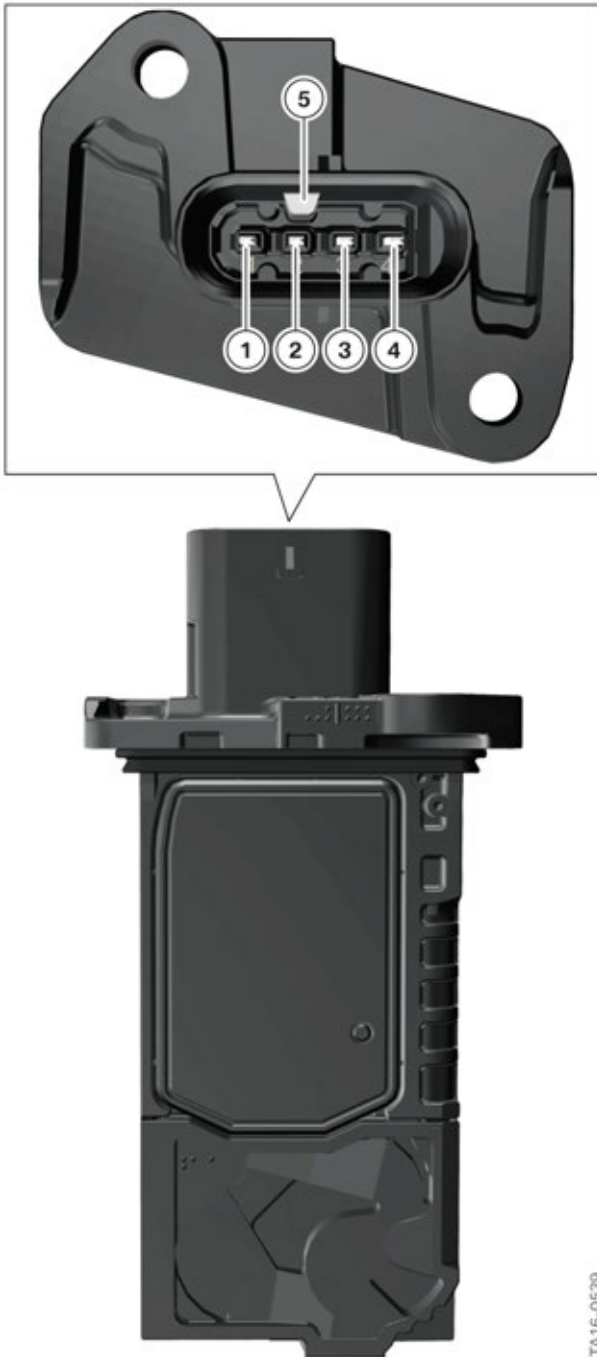
8th generation hot film air mass meter in the G30
