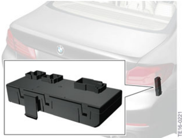
Trunk function module (HKFM)
