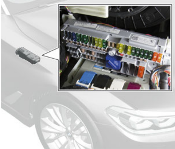
Power distribution box, front right
