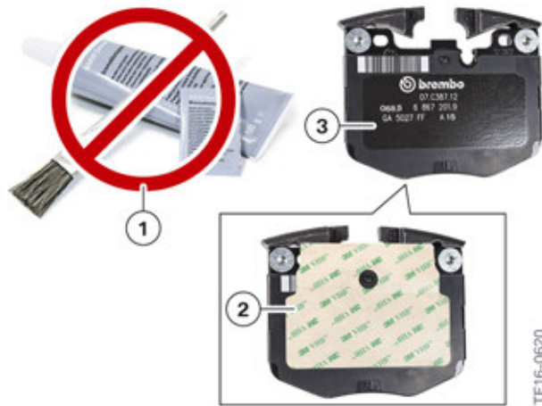
Bonded brake pad on the front axle of the G30
