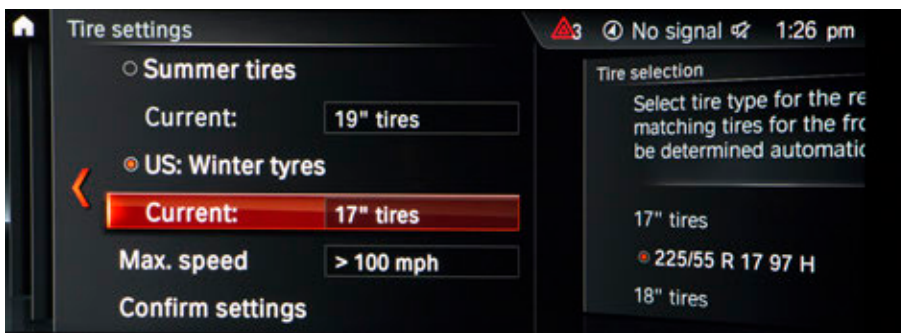
Adjustment of the tire sizes to be set on new wheels in the Central Information Display on the G30
