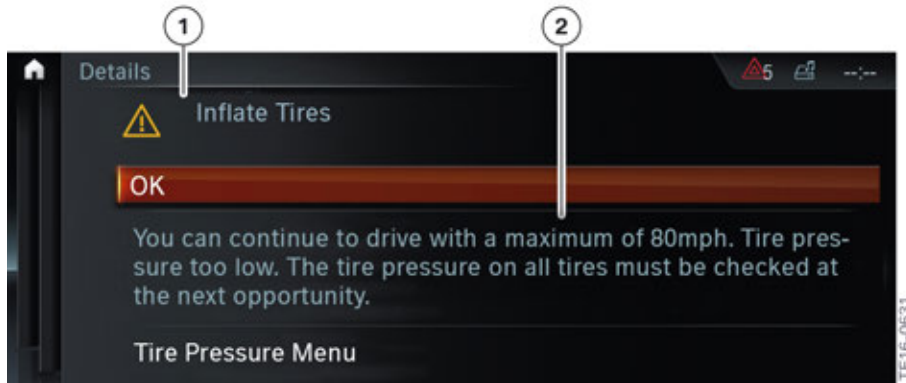
Warning level 2 Check Control message in the G30
