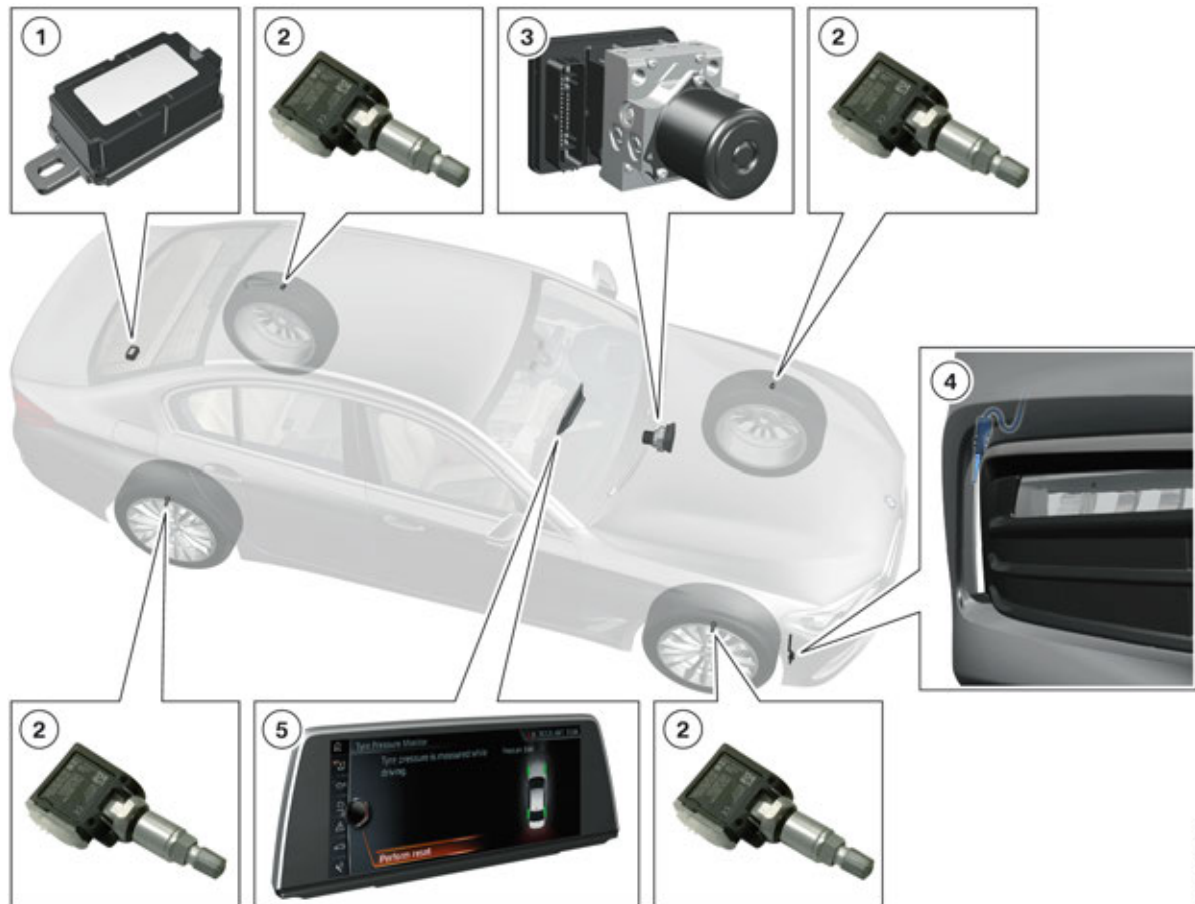
System overview of the electronic tire pressure label in the G30
