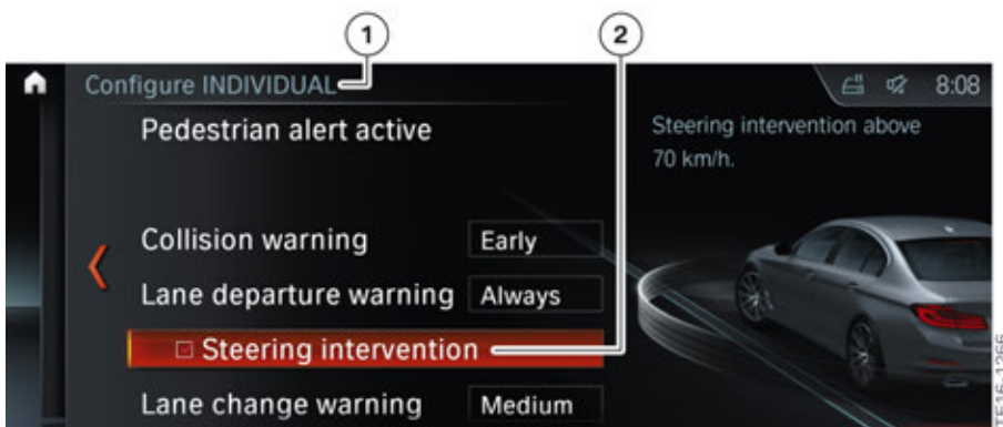
G30 Intelligent Safety view on the CID (Lane Departure Warning with active steering intervention)
