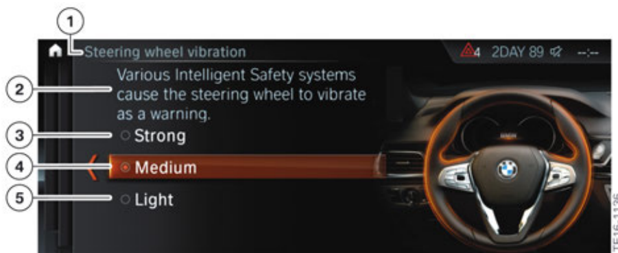
G30 Steering wheel vibration settings menu on CID
