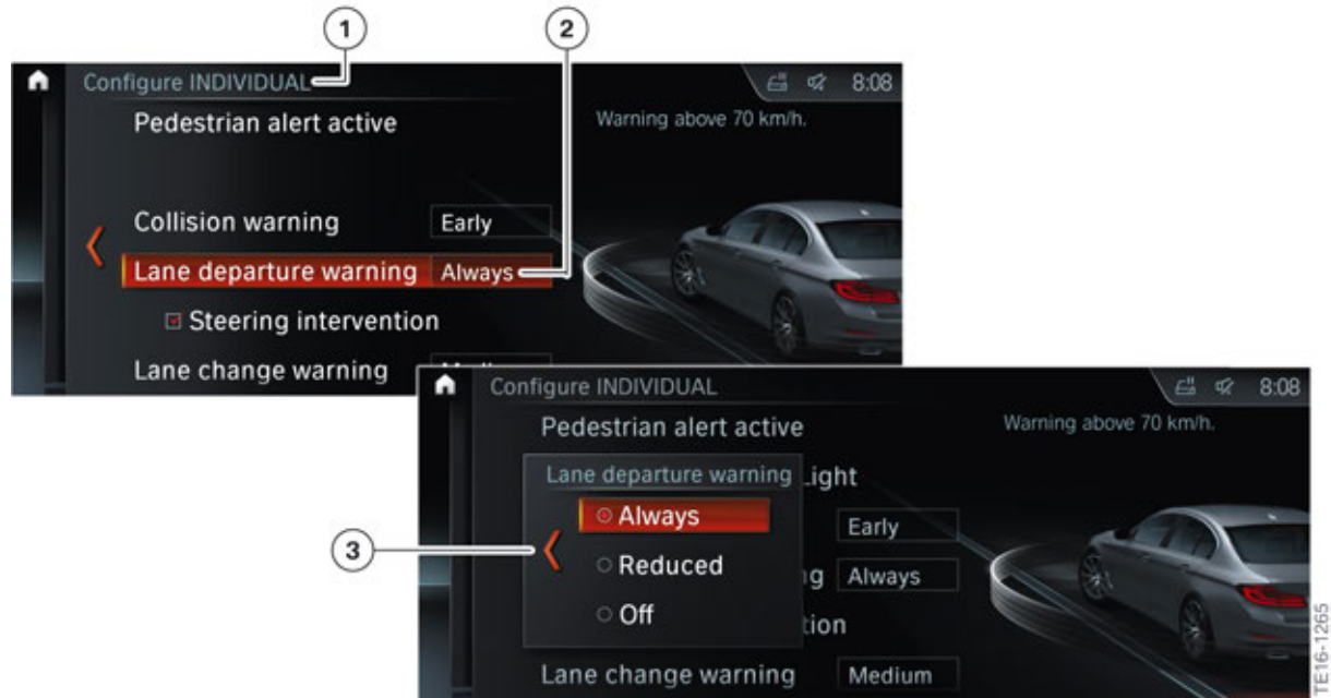
G30 Intelligent Safety view on the CID (Lane Departure Warning)
