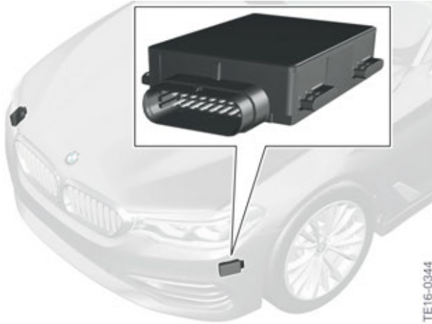
G30 Side Collision Avoidance (radar sensors)
