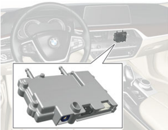
G30 Night Vision Electronics (NVE) control unit
