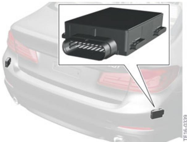
G30 Blind Spot Detection (SWW) (radar sensors)
