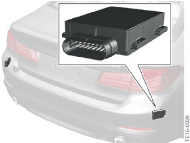
G30 Blind Spot Detection (SWW) (radar sensors)
