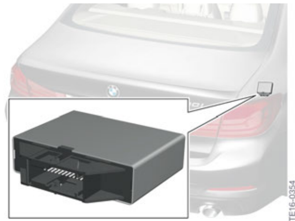
G30 Control unit for Parking Maneuvering Assistant (PMA)
