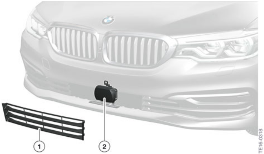
G30 Installation location of front radar sensor for ACC Stop&Go
