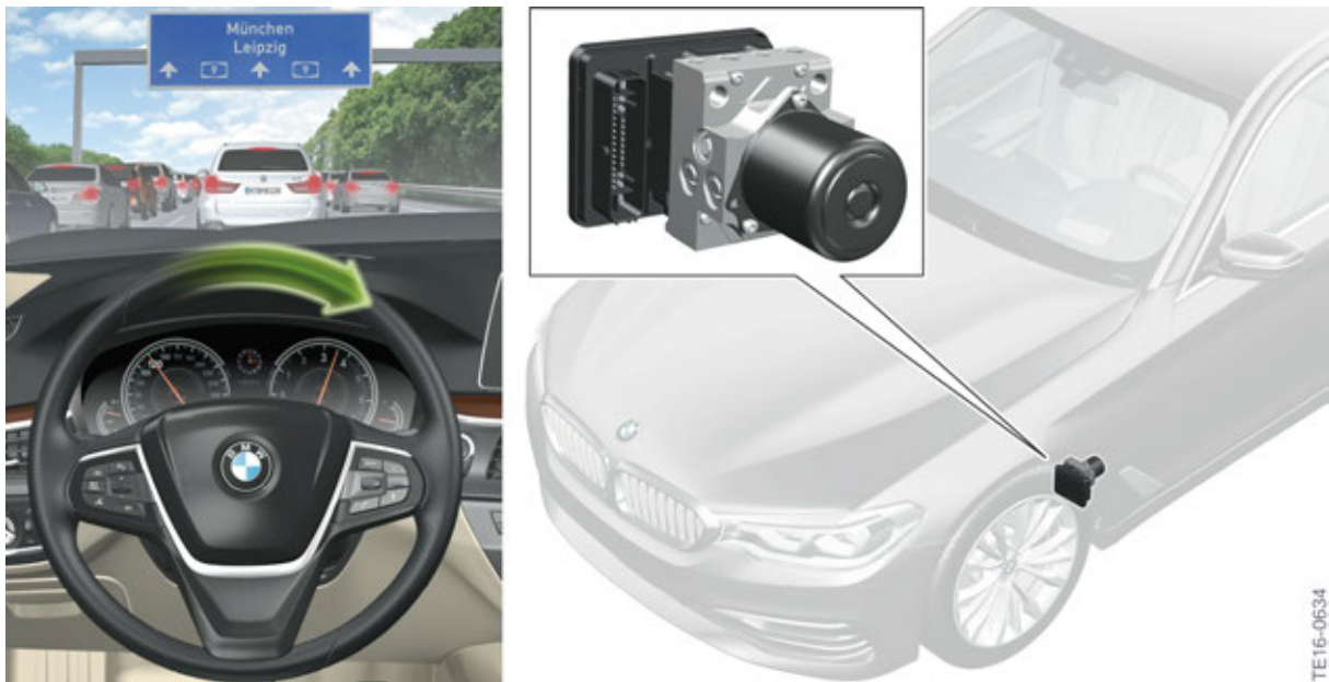
G30 Evasion Aid: interaction of Dynamic Stability Control( DSC) and Electronic Power Steering (EPS)
