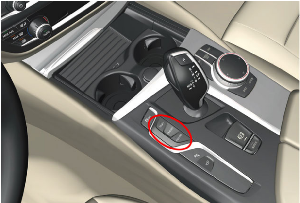
G30 Driving experience switch without the ADAPTIVE mode.
