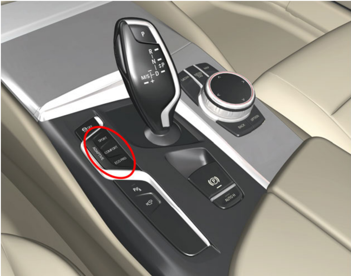
G30 Driving experience switch with the ADAPTIVE mode.
