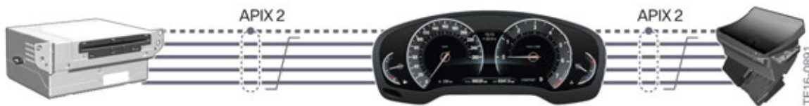
G30 Connection of the instrument cluster with the head unit
